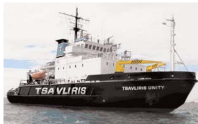
TS AVLIRIS Salvage Group has added a further salvage tug to its fleet. The new acquisition is the TS AVLIRIS Unity , built by Wartsila-Helsinki in 1983 as the Deimos . The tug, with a bollard pull of 85 tonnes, is now operating in the Indian Ocean region.
