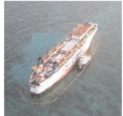
Titan Salvage successfully refloated the grounded ferry Arcangel in Cancun, Mexico, on July 1. The vessel – not in service at the time – was blown off its moorings last November. The salvage operation began in May and great care was exercised, as the vessel was very close to a reef inside a National Marine Park. Oil and waste water was discharged to a barge, the hull patched and ballast transferred prior to the refloating, achieved with the assistance of hydraulic pullers.
