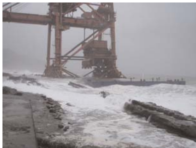
In early July Nippon Salvage successfully refloated the barge SHIN-35000 , laden with a 65 m tall, 2,500 tonnes gantry crane. The barge was under tow when the towline parted in rough seas off Miyazaki Prefecture at the beginning of June. The barge suffered heavy bottom damage but was refloated by air injection and towed into Aburatsu Port .
